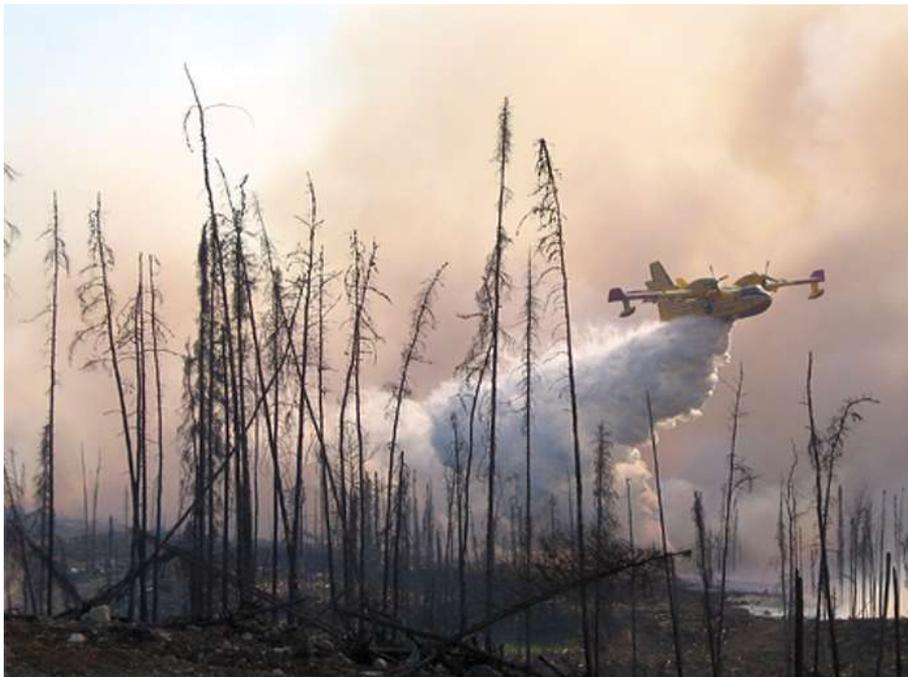
**CL-415 Heavy Water Bombers:** CL-415 is a Canadian-built amphibious aircraft built specifically for aerial firefighting. The CL-415 can scoop up to 6,130 litres of water from a nearby water source and drop it on a fire..
